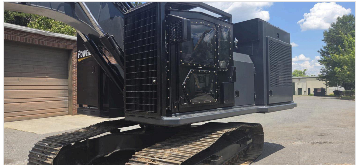
New heavy-duty XPE cab – roll cage + polycarbonate windows
