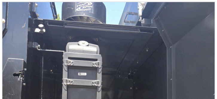
Heavy-duty precleaner ahead of the air filter
